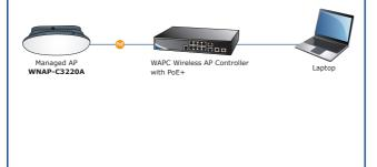
Step 3: Launch the Web browser to log in to the WAPC Wireless AP Controller Web pages. Configure the Wireless setting for the WNAP-C3220A under "AP Control".
